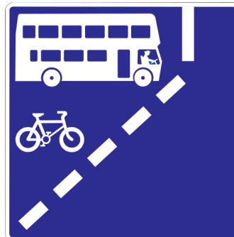
Advance sign for with-flow bus lane
